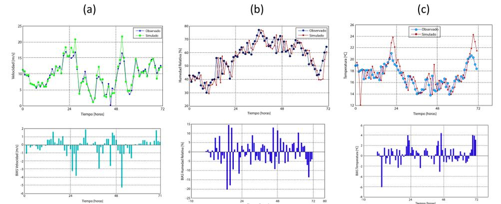
**Figure 5.** Upper panel: Hourly evolution of (a) wind speed (m/s), (b) relative humidity (%) and (c) temperature (°C) at wind turbine location (17.6294°S y 65.2841°W, 80 m above surface level) over the forecast period (16-18 October 2015) : bias-corrected WRF forecast (green and red) and registered values at the meteorological station (blue). Lower panel: Hourly evolution of the corresponding forecast errors.
