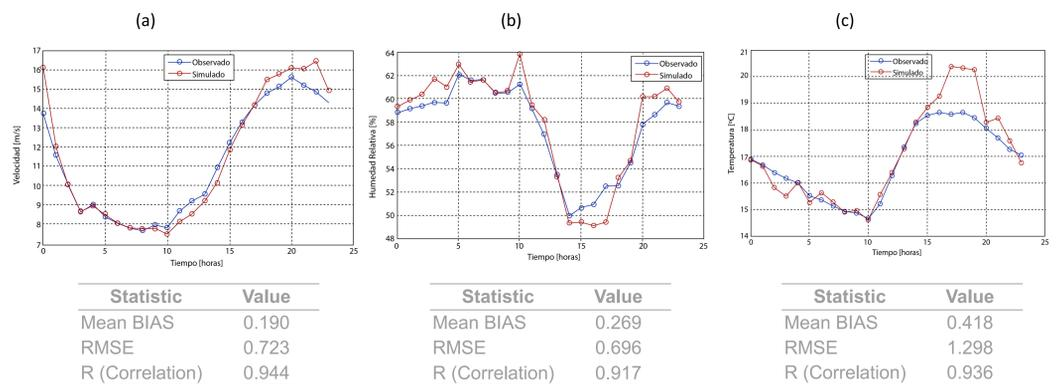
**Figure 4.** Mean diurnal cycle of (a) wind speed (m/s), (b) relative humidity (%) and (c) temperature (°C) at the wind turbine location (17.6294°S y 65.2841°W, 80 m above surface level) over the forecast period (16-18 October 2015) : bias-corrected WRF forecast (red) and observations from the meteorological station (blue). The corresponding validation statistics are indicated below each plot.
