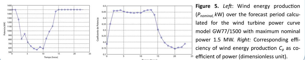
**Figure 5.** Left: Wind energy production ( $P_{nominal}$ , kW) over the forecast period calculated for the wind turbine power curve model GW77/1500 with maximum nominal power 1.5 MW. Right: Corresponding efficiency of wind energy production  $C_p$  as coefficient of power (dimensionless unit).
